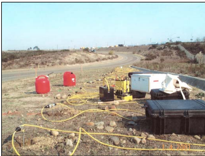
Figure 1 – Sting Resistivity Imaging System.
